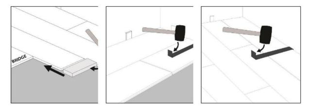
Step 7: Tap end of plank with hammer and tapping block to lock ends of planks together. Remove bridge and continue towards wall until installing the final plank in the row. BE SURE TO TAP ON EDGE OF RIGID SO AS NOT TO DAMAGE LOCKING PROFILE.
