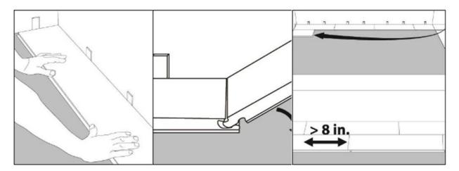
Step 1: Begin installation working from left to right. Insert spacers at ends and edges where planks meet wall.
