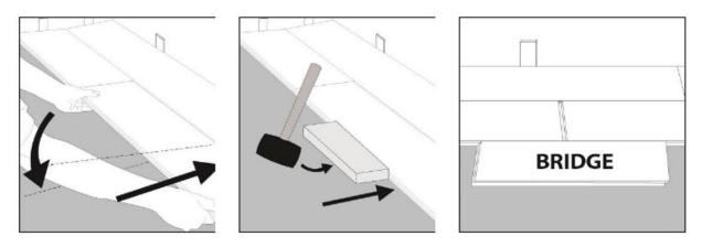
Step 4: Lock long edge of plank by inserting tongue into groove at an angle and drop in place. Slide plank toward end of previously installed plank until the tongue just touches the groove.
